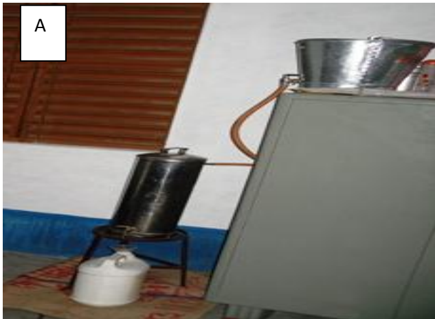
Figure 4: A. Fluoride Filter Unit Installed in Field B. Experimental Result of Cumulative Volume of Water Treated versus Outflow Fluoride Concentration
